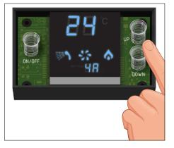
Select UP / DOWN to set the correct fan speed (Refer to FL value in table)
