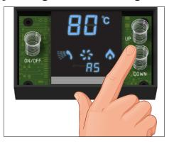
Select UP / DOWN to alter parameters until the manometer gives appropriate value (Refer to PH value in table)
