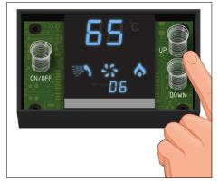
Select UP / DOWN to set the correct fan speed (Refer to FH value in table)
