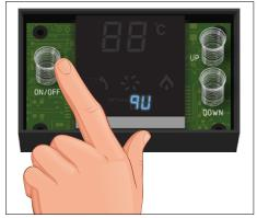
Press ON/OFF to confirm all changes (Controller will beep four times to confirm)
