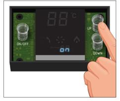
Select UP to set unit to 70°C (On) Select DOWN to set unit to 50°C (Off)
