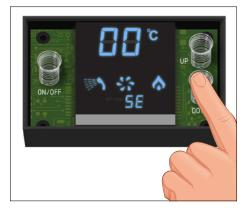
Select UP / DOWN to alter parameters until the manometer gives appropriate value (Refer to dH value in table)
