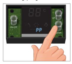
Press and hold DOWN for 3 seconds within 3 seconds of power being turned on to the unit.
