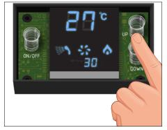
Select UP / DOWN to alter parameters until the manometer gives appropriate value (Refer to PL value in table)
