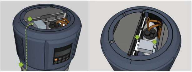
Wire electrics by feeding the cable through the access hole on the under face of the upper section of the unit and up to the electrical compartment. Remove electrical compartment cover by releasing the two screws & wire accordingly. (Where possible terminating the electrical connection with a suitable isolating switch (By authorised electrician)
