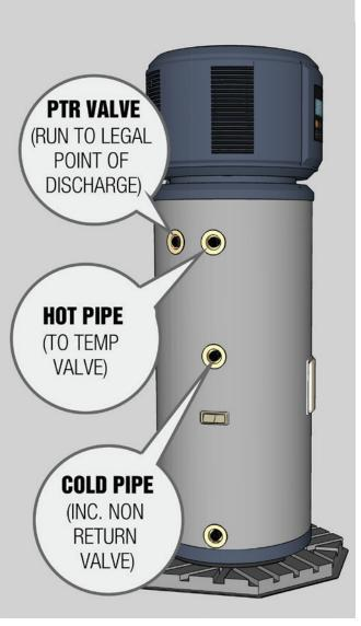
Connect the hot pipe, the cold pipe (ensure non-return valve is used at the tank location) & connect PTR valve (drain to legal point of discharge)
