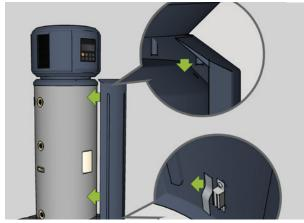
Fit the fascia cover using the locating pins at the top & magnet at the lower position (for successful fit ensure protective tape on the magnet is removed)
