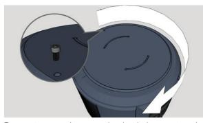
Remove top cover (to access the electrical compartment) by removing the locking screw and rotating in a clockwise direction. Simply lift up to remove and put aside.
