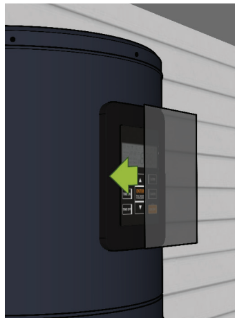
Fit UV Screen shield to the control panel
