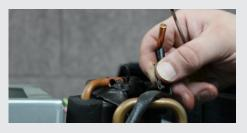
Continue by removing the cable tie holding the sensor in place and then remove the sensor. Inspect for any visual damage to the sensor and its lead and check that the corresponding connector is securely seated in the TP socket on the PCB.
