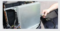
Check the connection between the display PCB and the mother PCB for any loose connections or cable damage.
