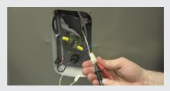
Simply release the corresponding connector and test for the appropriate resistance using a multimeter. The resistance reading will vary depending on the temperature within the tank so you will need to confirm the correct reading by referring to the resistance chart. (Click to open chart). If you are receiving a suitable reading, reconnect the connector and ensure this is securely in place.
