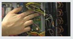
If you are not receiving a suitable reading, access the PCB board and check the corresponding connector is securely connected to the PCB in socket T5L. Once the connector has been checked, retest resistance.
