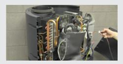
Once the screws are removed carefully pull the front casing away enough to access the controller connector and release. Then put the front casing aside.
