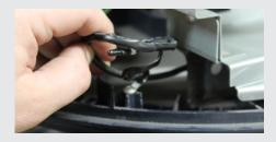
To remove sensor, simply unwind the holding clip / wire until the sensor is clear. Inspect for any visual damage and check that the corresponding connector is securely seated in the T4 socket on the PCB.
