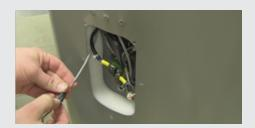
If this continues to provide an unsatisfactory reading, remove the sensor by turning counter clockwise and pulling directly away from the tank.
