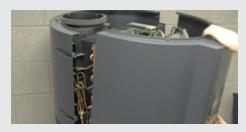
If the controller is indicating an error of E2, then there is an issue with the connection between the display PCB and the mother PCB.
