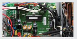
If you are not receiving a suitable reading, access the PCB board and check the corresponding connector is securely connected to the PCB in socket T5. Once the connector has been checked, retest resistance.
