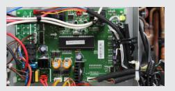
Then to release the sensor, cut the cable tie and gently pull down out of it's container. Inspect for any visual damage to the sensor and its lead and check that the corresponding connector is securely seated in the TH socket on the PCB.
