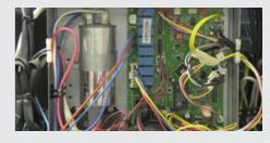
If there is still no voltage at the manual thermostat then check the UE connector within the electrical compartment is providing power.
