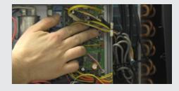
If you are not receiving a suitable reading, access the PCB board and check the corresponding connector is securely connected to the PCB in socket T5U. Once the connector has been checked, retest resistance.
