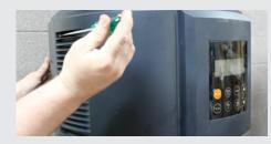
Then lift the top cover up and put aside. Then release the four fasteners, two either side holding the front casing on.
