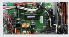
If there is still no voltage at the thermostat then check the UE connector within the electrical compartment is providing power.
