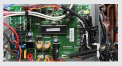
If there was no voltage at the thermostat then check the UE connector within the electrical compartment is providing power.
