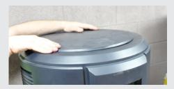
Remove the screw from the top cover (on the top face at the rear), then rotate the top cover counter-clockwise to release
