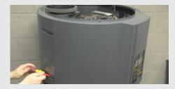
Then release the four fasteners, two either side holding the front casing on.
