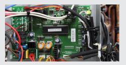
If it appears the sensor needs replacing, disconnect the T3 connector at the PCB location and feed the cable through to the sensor location.
