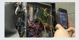
If the E8 error is presenting on start up, then we need to inspect a few items within the electrical compartment. Firstly check that all connectors are securely seated in there corresponding socket. Perform an inspection across the electrical compartment checking for any damage or signs of moisture.
