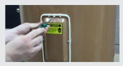
If the controller is indicating an P8 error, then there is an issue with the circuit of the E-heater To assess this error, proceed to access the element compartment located in the lower compartment under the front fascia cover. Remove the lower electrical cover by removing the array of screws and put cover and fasteners aside.
