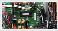
If the E8 error is presenting on start up, then we need to inspect a few items within the electrical compartment. Firstly check that all connectors are securely seated in there corresponding socket. Perform an inspection across the electrical compartment checking for any damage or signs of moisture.
