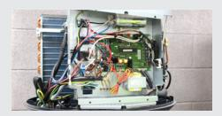
At this time it is also recommended to open the electrical compartment which is located directly behind the control panel. To access simply remove the compartment panel by removing the two lower screws & two upper screws.
