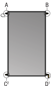
Single Collector (Panel) System with frost valve
